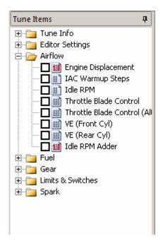
When using the compare feature, a colored flag may be visible next to certain tune items. These visual identifiers helps you distinguish parameters that don't match when using the compare feature. Visual identifiers offer a quick and easy way to identify where the tune has changed.
