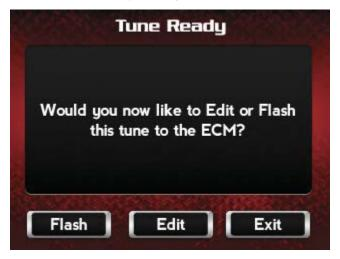
**Note:**You can edit any tune that's loaded in the Tune Manager prior to flashing your ECM. The Power Vision allows you to make basic adjustments to your tunes directly on the device without using a computer. In order to gain full access to your tune files, you'll need to download them from the Power Vision to WinPV, our custom tuning software.
