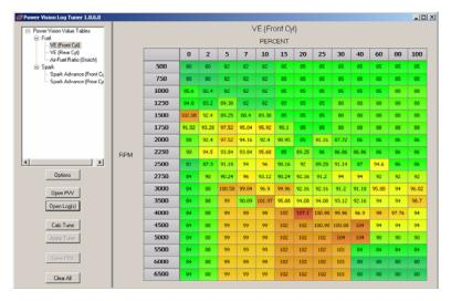
7 In the Log Tuner tree, click **VE Delta** for both the front and the rear cylinder.
