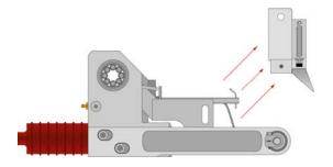
2) Holding the Tooling Head remove the clamp release screw and remove head assembly.
