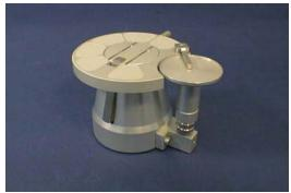
**Non Heated Work holder**: Non-rotating work holder for substrates up to 1.000" x 1.000". Work piece is held by mechanical clamp, with 2 Position, 2.000" x 2.000" fluoroware supports. Assembly No. 3600.220.
