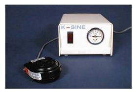
**K~1311 Vacuum Flow Control:** The operator, by means of an Off/On footswitch, can disengage the vacuum to the work area releasing the part to replace with another. A vacuum gauge on the front of the control box displays the pressure in inches of Mercury.
