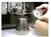
This option allows the operator to calibrate the "Force" setting by simply adjusting the force adjustment knob. This black plastic knob  $\leftarrow$  is located directly to the right of the tooling head. To increase the bond force turn the knob counter-clockwise. To decrease the bond force turn the knob clockwise. Measure the force by placing a gram gauge just in front of the bond tool and lift until the machine beeps. Repeat to verify force is correct.
