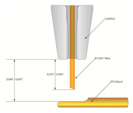
The above drawing represents the recommended setup for 0.001" wire. These numbers are approximations and may vary for different applications.
