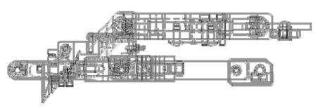
transducer uses a bond tool of 0.750" length dropped 0.65625" below center. Vertical clearance is a full 0.375" everywhere under these tool heads and all other mechanism except for wire presentation at 45° for angled feed. Wire Clamps are air-opened and spring-closed, and have self-contained closure pivots. A
