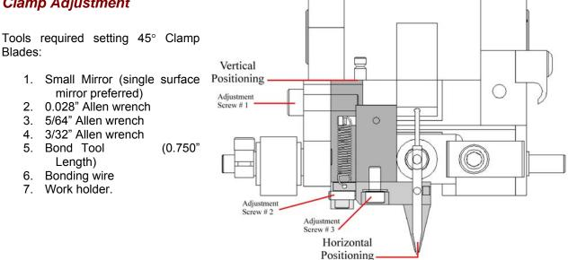
The following procedure is for setting the 45-degree clamp blades. When adjusted properly the clamps will feed the wire through the bond tool straight, leaving the wire tail directly under the bond foot for all subsequent bonds.
