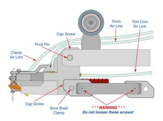
**5)** Bring the FORCE STRUT ARM up and slide the STRUT SHAFT through the mounting hole and clamp the shaft by tightening the Dutch Key. Locate the air lines for the clamps and the torch and connect them to their respective hose barbs on the front panel. Plug in each of the connectors (3 total) into the sockets on the front panel. Finally, change the machine model number as described below.
