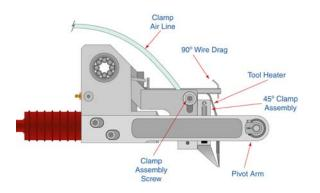
1) Remove the **bonding tool**. Disconnect the Clamp Air Line from the front cover panel and the small clamp securing the hose to the side of the head assembly. (Enter the Edit Sequence so that the machine will not fire ultrasonics when the head is being moved around).
