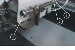
To adjust the low force setting, loosen the knurled lock nut  $\uparrow$  and turn the adjustment knob  $\rightarrow$  located behind
