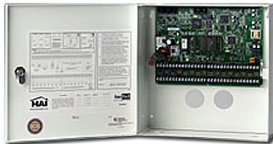
Controller and PIM
