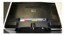
Take a look at the neck that's connecting the base to the TV. There should be 4 screws on the neck and 2 screws on the side. Remove the 6 screws and the base will slide off.
