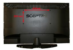
Mounting Specification : **400mm x 200mm** using screw size **M6**. Length of screw should not exceed **12mm**. Please Note : The **12mm** length of screw refers to how deep the screw can go inside the mounting holes. When you're buying screws, you should add the original 25mm to the thickness of your mounting plate in order to get the total screw length.
