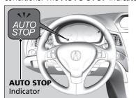
The engine then restarts once the vehicle is about to move again, and the indicator goes off.
