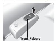
Pulling the trunk release to the lower left of the driver's seat unlocks and opens the trunk.
