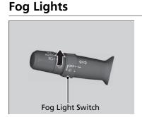
When the low beam headlights are on, turn the fog light switch on to use the fog lights.
