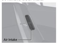
If the air intake is obstructed during vehicle operation, the IMA battery can become too hot. To protect the battery, the system may start limiting IMA battery output power and cause the Acura hybrid system and 12 volt battery charging system indicators to come on.
