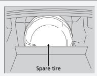
The spare tire is stored at the back of the trunk, behind the rear seat-backs.
