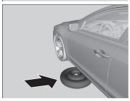
**8.** Place the compact spare tire (wheel side up) under the vehicle body, near the tire that needs to be replaced.
