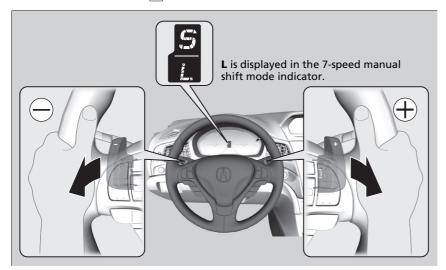
To cancel this mode, pull and hold both paddle shifters again, or move the shift lever from  $\fbox{S}$  to  $\fbox{D}$ . The  $\r{L}$  indicator goes off.
