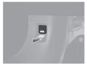
Locate the hood latch lever, slide the lever and lift up the hood.
