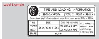
This figure includes the total weight of all occupants, cargo, and accessories, and the tongue load if you are towing a trailer.
