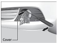
**2.** Insert a flat-tip screwdriver into the tab at the inside edge of the cover, then pull straight out as indicated to remove the cover.
