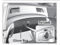
Pull the handle to open the glove box. You can lock the glove box with the built-in key.
