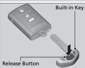
The built-in key can be used to lock/unlock the doors when the keyless access remote battery becomes weak and the power door lock/unlock operation is disabled.
