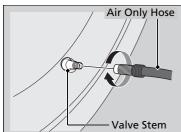
**5.** Attach the air only hose onto the tire valve stem. Screw it until it is tight.
