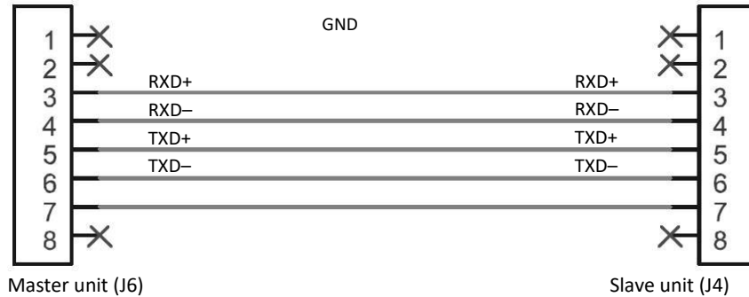
Figure 5-6 RS-485 Communication Cable from Master to Slave Unit
