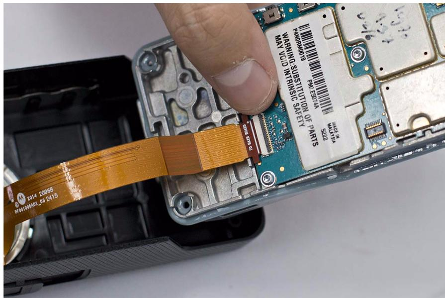
Figure 5-9. Disconnecting the UC-audio flex (Non Keypad Model)
