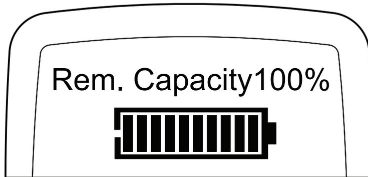
Figure 3-2. Battery Check Test Mode Display
