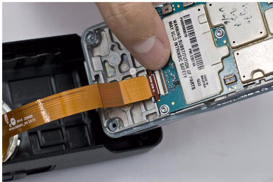
Figure 5-40. Interface flexes reassembly (Non Keypad Model)
