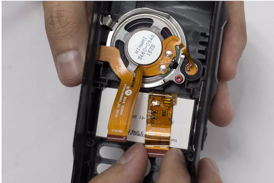
*Figure 5-29. Display module reassembly*
