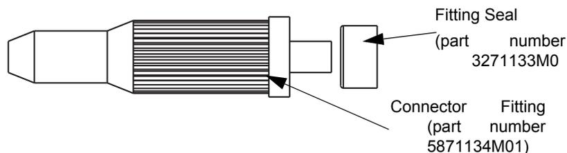
Figure 5-47. Connector Fitting - Fitting Seal Pump Connector
