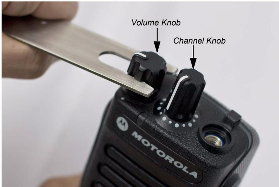
Figure 5-4. Volume and Channel Knob removal.
