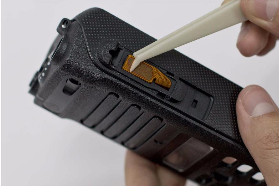
*Figure 5-20. UC-audio flex removal*
