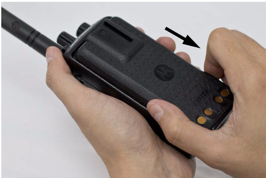
*Figure 5-2. Battery removal*
