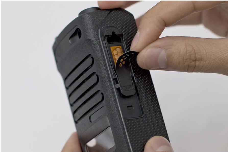
*Figure 5-19. UC escutcheon removal.*
