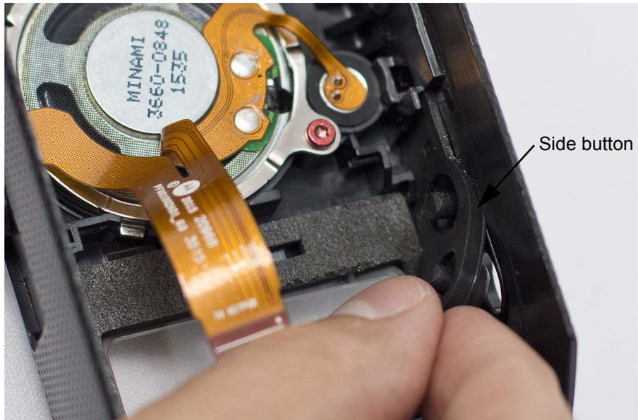
Figure 5-27. Side button reassembly
