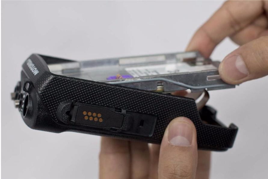
*Figure 5-41. Front kit reassembly*
