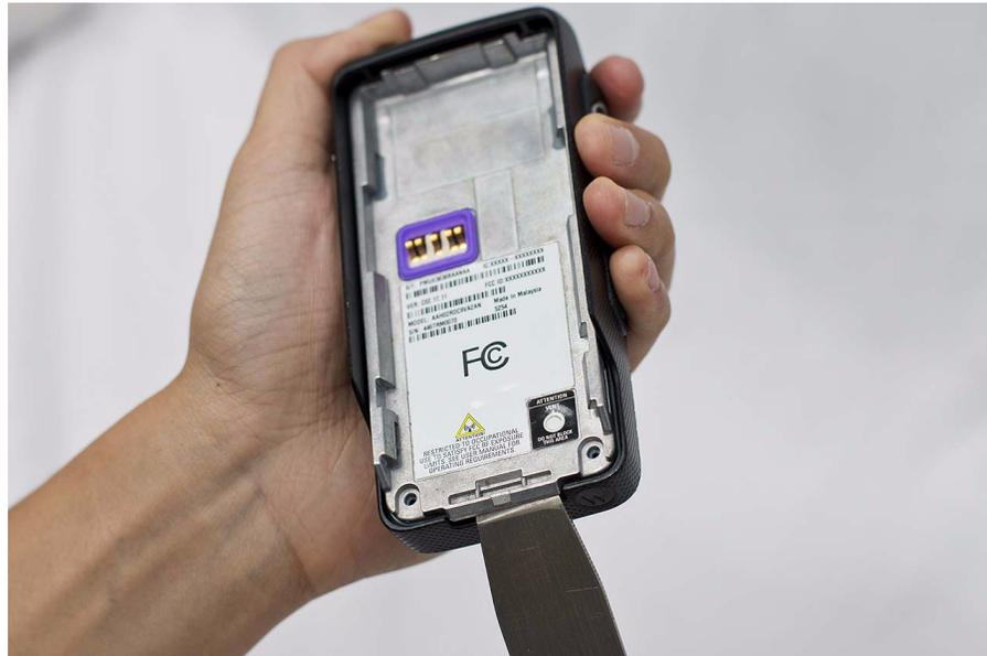
Figure 5-6. Back Kit disassembly
