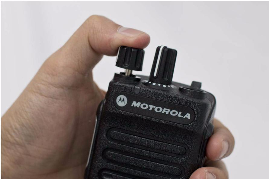
*Figure 5-42. Knob reassembly*
