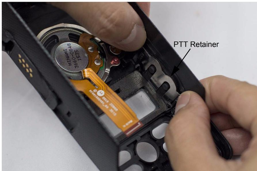
Figure 5-28. PTT retainer reassembly
