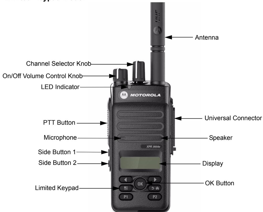
Figure 1-1. Limited Keypad Model
