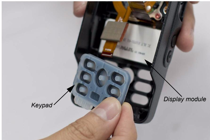
*Figure 5-16. Keypad removal*
