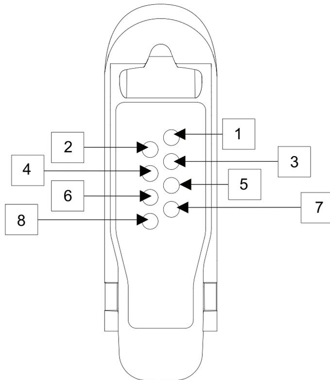
Figure 2-2. Pin Layout of Side Connector
