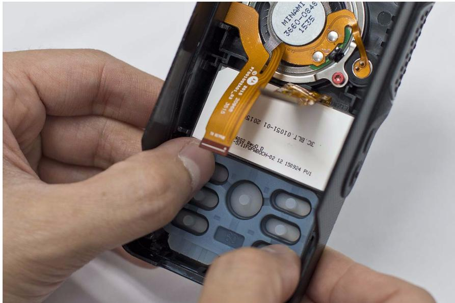
*Figure 5-30. Keypad reassembly*
