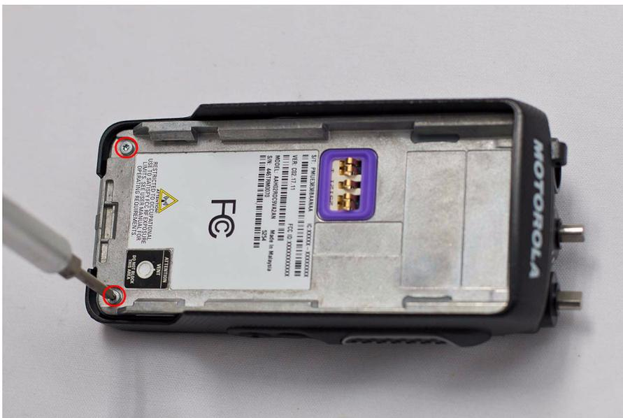
Figure 5-5. Front Kit-Back Kit Screw removal
