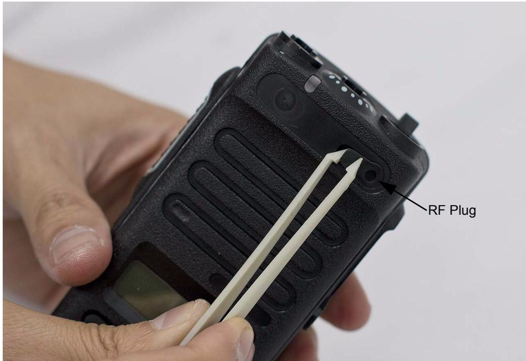
*Figure 4-3. RF Plug disassembly*
