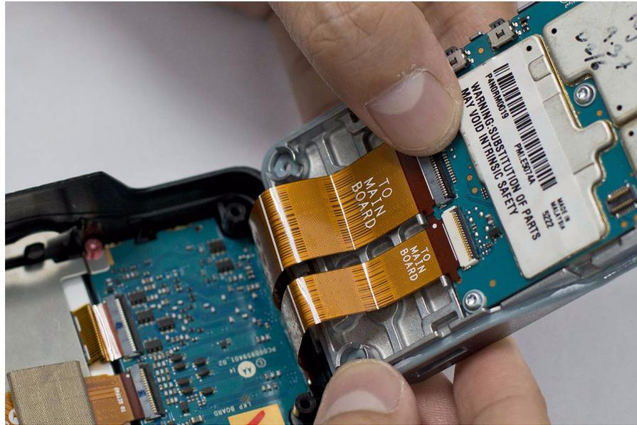
Figure 5-39. Interface flexes reassembly (Limited Keypad Model)
