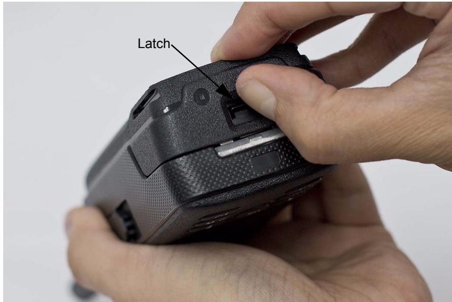
*Figure 5-1. Battery removal*
