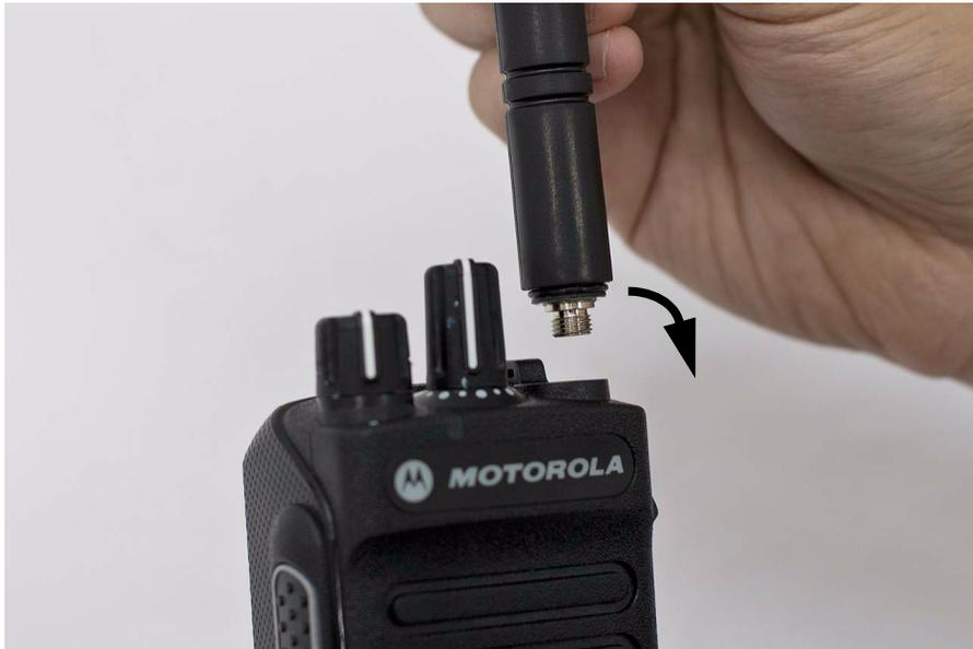
*Figure 5-43. Attaching the antenna*
