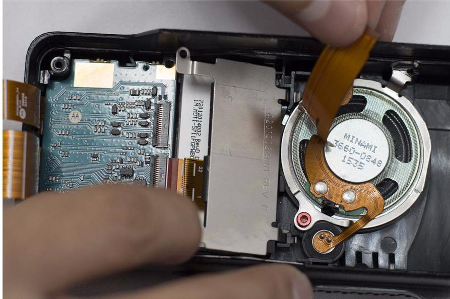
Figure 5-33. Speaker retainer reassembly
