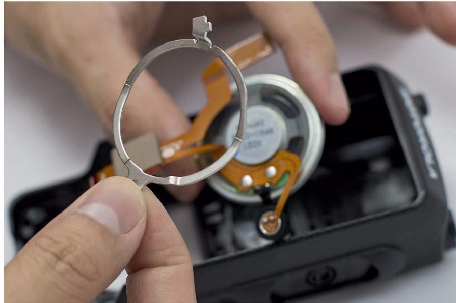
*Figure 5-22. Speaker retainer removal*
