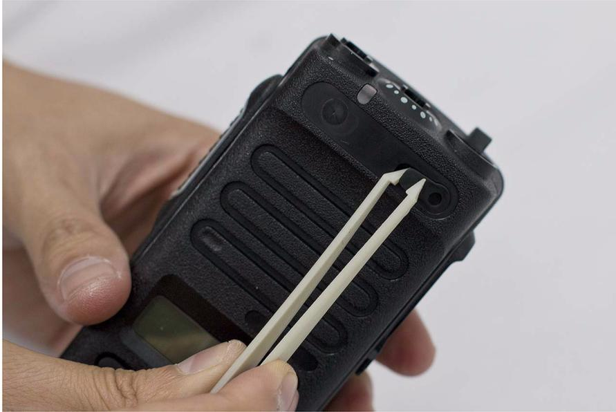
*Figure 5-44. RF Plug reassembly*
