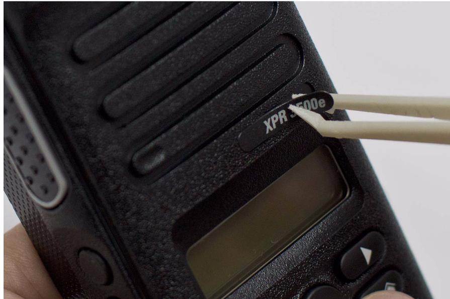
*Figure 5-46. Product Nameplate Reassembly*
