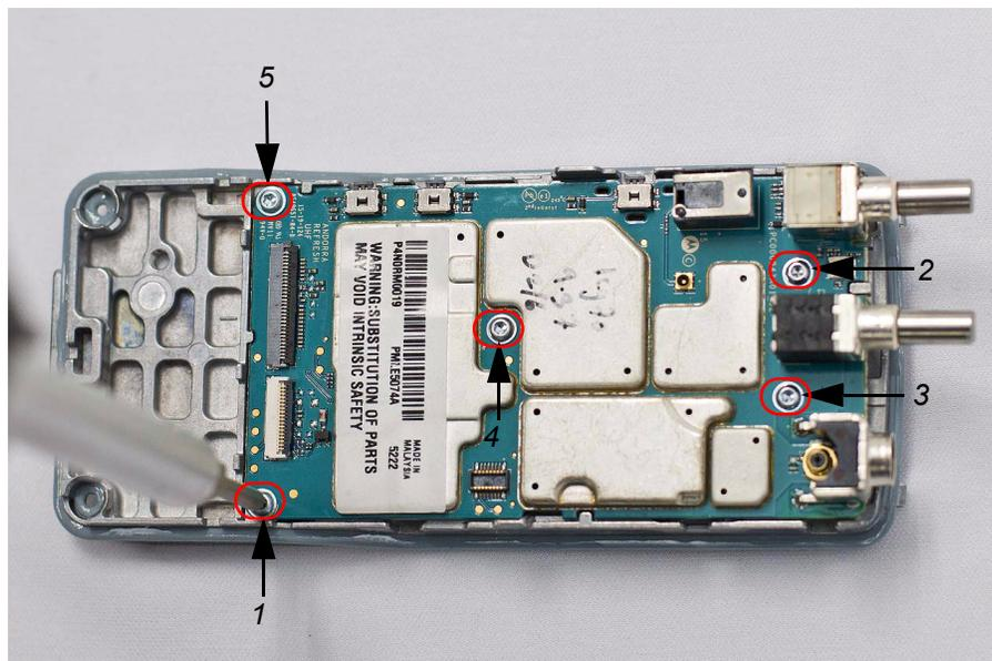
Figure 5-37. Mainboard reassembly
