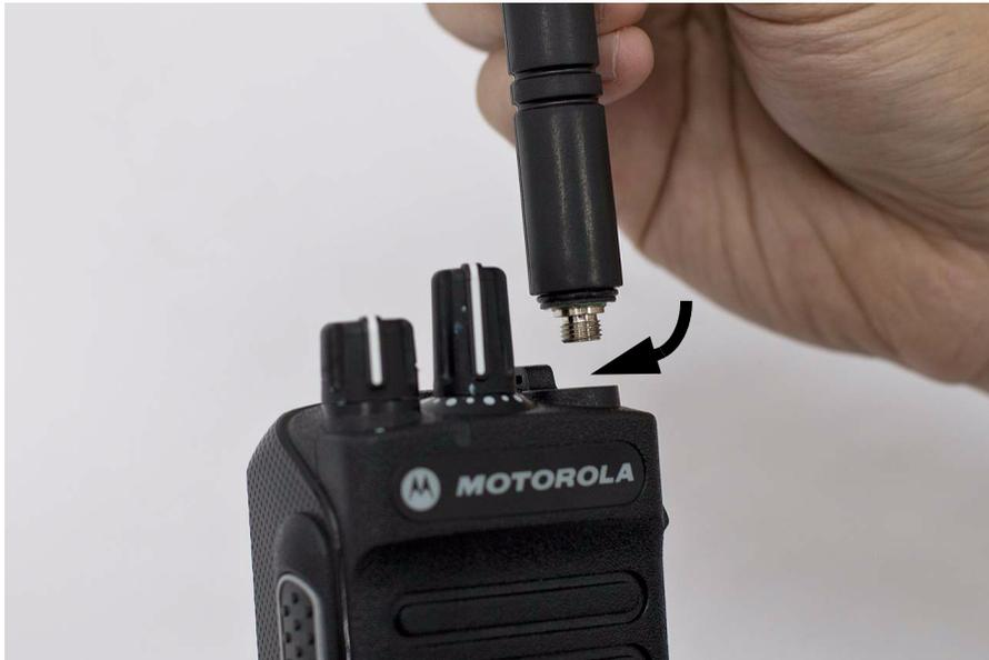
*Figure 5-3. Antenna removal*
