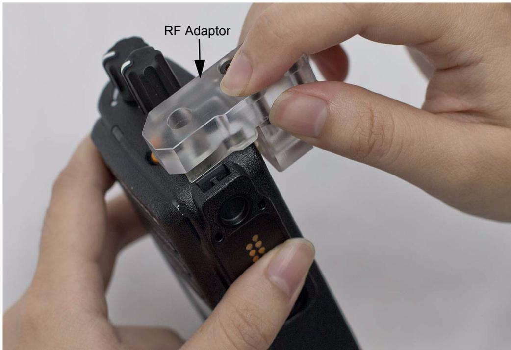
*Figure 4-4. RF Adaptor insertion*
