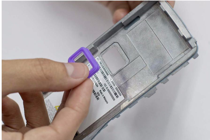
*Figure 5-12. Battery contact seal removal*
