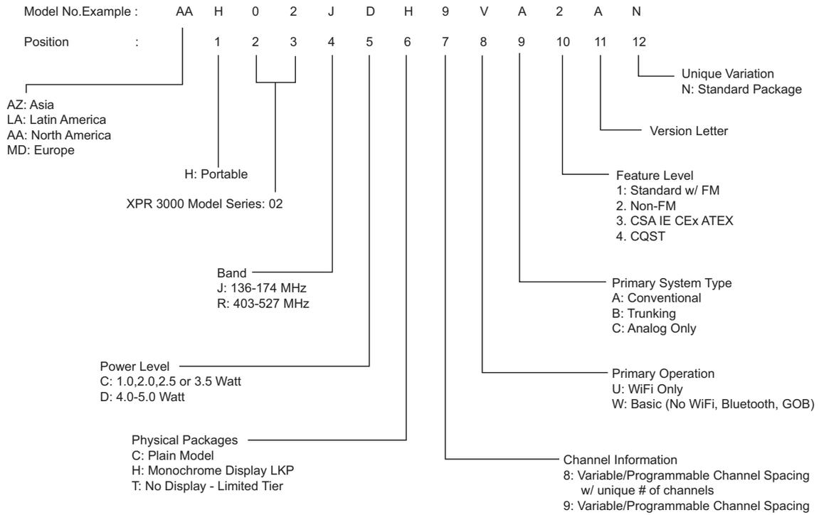
Figure 1-3. Portable Radio Model Numbering Scheme
