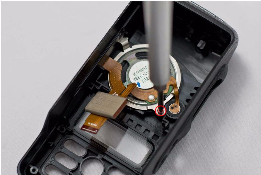
*Figure 5-21. Speaker retainer screw removal*
