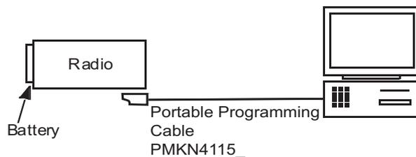
Figure 4-1. CPS Programming Setup
