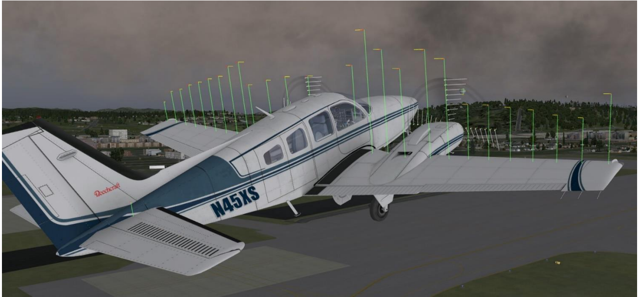
Figure 5.7: Illustrating the forces acting on a Baron 58
