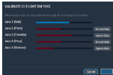
Figure 4.2: The calibration window of the Joystick settings screen, with the device partially calibrated
