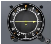
Figure 7.2: The ADF in the Cessna 172
