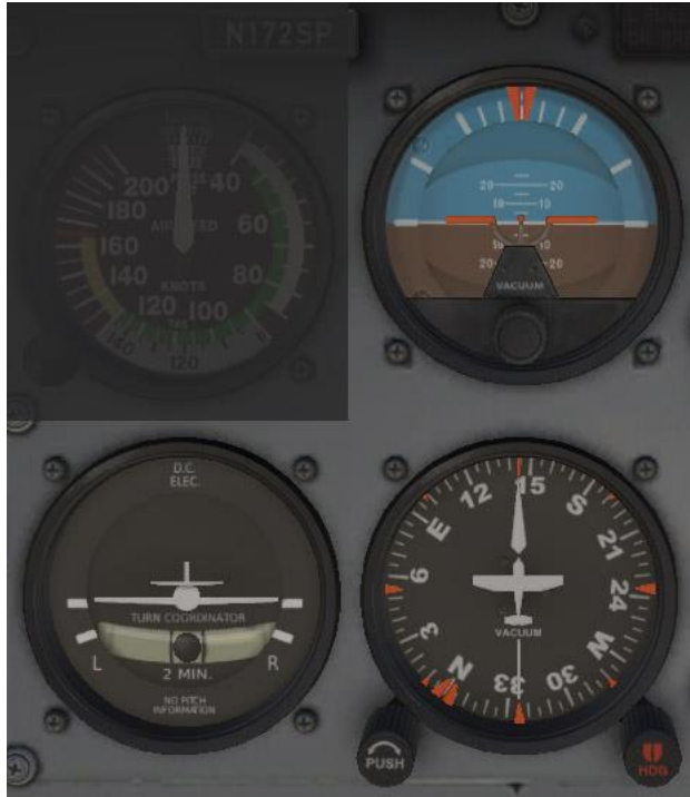
Figure 7.5: The three primary gyroscopic instruments in the Cessna 172
