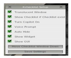
The "Xchecklist Setup" dialog box will be explained first and can be found by clicking on the Plugins menu item and selecting Xchecklist from the drop down list.
