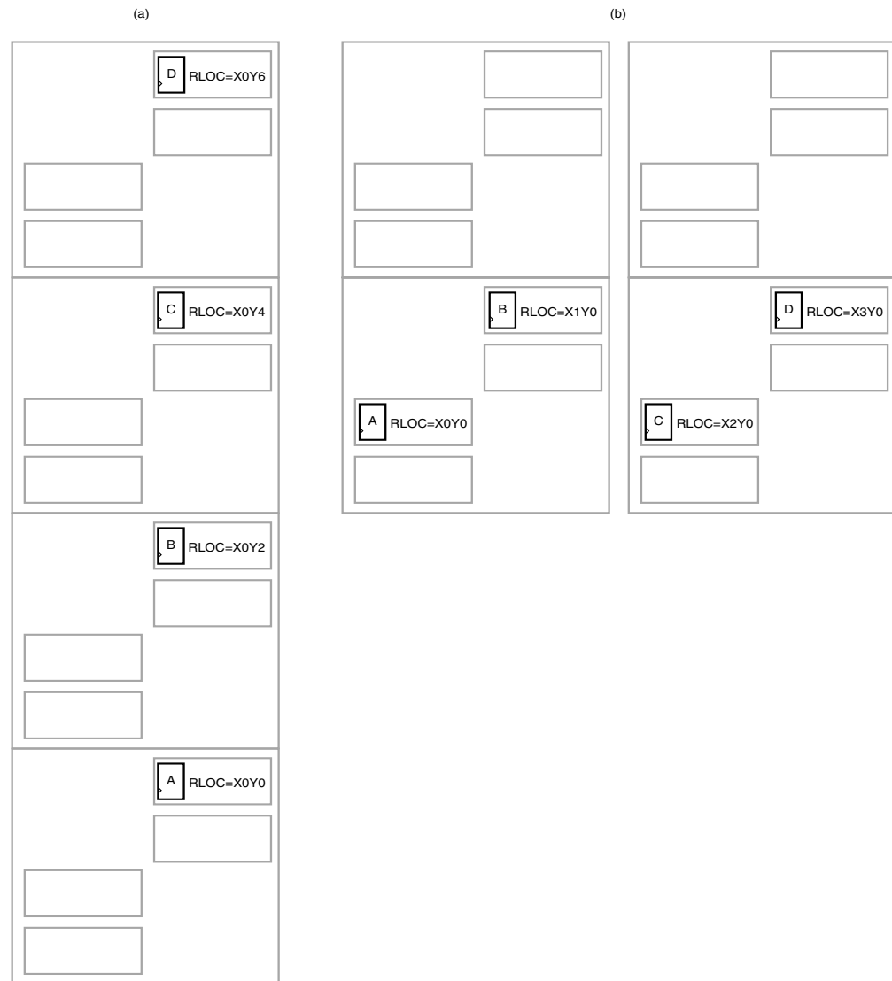
Figure 70-2: Different RLOC Specifications for Four Flip-Flop Primitives
