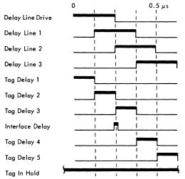
Timing Chart is shown for Address In or Select In Conditions.
