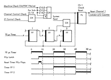
Figure 3B-78. Channel Reset by Machine Check
