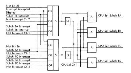
Figure 3B-40. CPU Subchannel Select and Interrupt Priority
