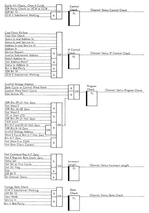
Figure 3B-34. Channel O Check Latches
