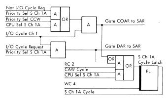
Figure 3B-12. Subchannel Cycle Latch
