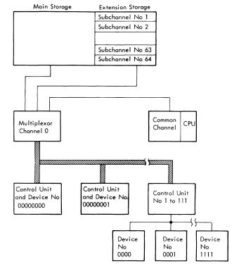
Figure 3B-13. MPX Channel 0 Data Flow Block Diagram
