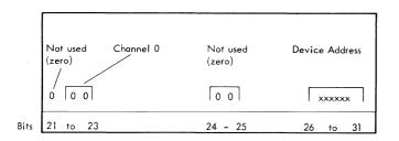
Figure 3B-18. Single Subchannel Address Format
