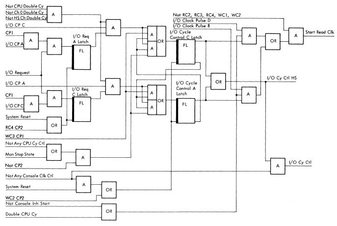
Figure 3B-8. I/O Cycle Request Latches
