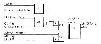
Figure 3B-73. Incorrect Length Latch
