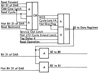
Figure 3B-54. Gating of B2 Buffer Register to Data Register
