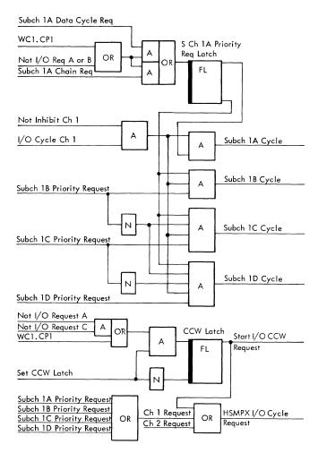
Figure 3B-7. HSMPX Channel I/O Cycle Request
