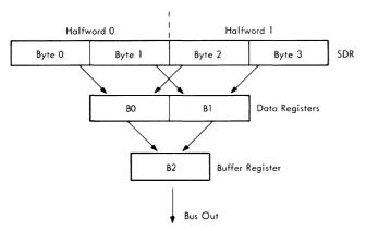
Figure 3B-58. Data Flow (Write)
