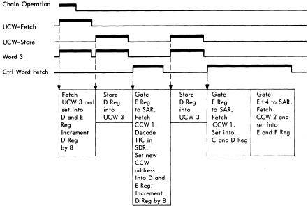
Figure 3B-28. Transfer-in-Channel Sequence
