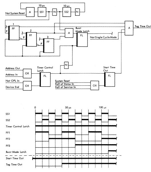
Figure 3B-44. Burst Mode and Tag Time Out
