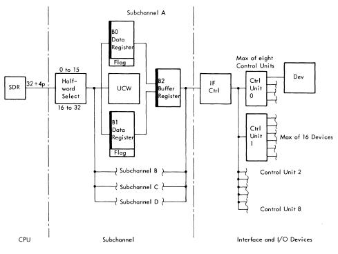
Figure 3B-35. HSMPX Simplified Channel Data Flow
