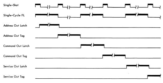
Figure 3B-46. Single-Cycle Timing for Initial Selection (Service-In)
