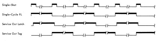
Figure 3B-47. Single-Cycle for a Burst-Mode Operation (Service-In)
