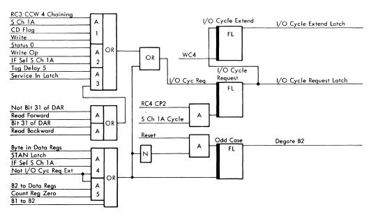
Figure 3B-55. I/O Cycle Request and Extend Latches
