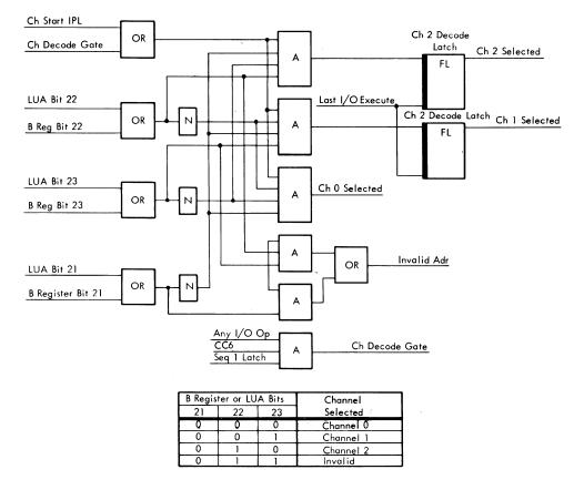
Figure 3B-3. Channel Decoding
