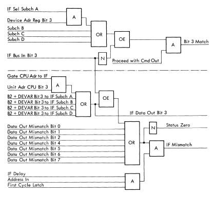
Figure 3B-42. IF Address Match, Status Zero and Bit 3 Match
