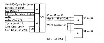
Figure 3B-61. Gating of Data Registers to B2 Buffer Register
