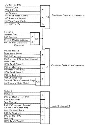
Figure 3B-32. Channel 0 Condition Code Generation
