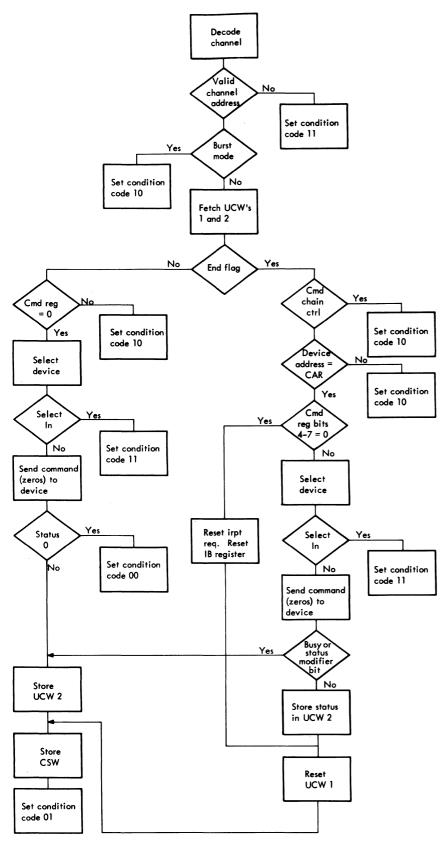
Figure 3B-30. Test I/O
