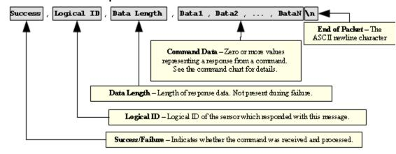
When an ASCII command is called wirelessly, before the data it would normally return in wired mode, it will return status values, each seperated by a comma. First is the **success/failure value**, which is a 0 if the command was successful and 1 if it was not. Some things which can cause a failure are:
