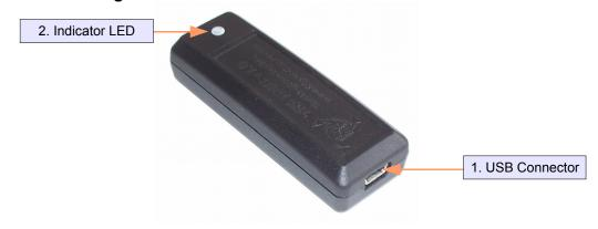
1. USB Connector – The 3-Space Wireless Dongle uses a 5-pin mini USB connector to connect to a computer via USB. The USB connector provides for both power and communication.
