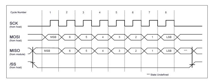
The diagram and parameter table below illustrates additional timing requirements and limits of the SPI interface:
