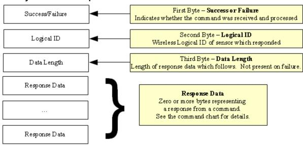
When a binary command is invoked wirelessly, before the data it would normally return in wired mode, it will return status bytes. First is the **success byte**, which is a 0 if the command was successful and non-0 if it was not. Some things which can cause a failure are:
