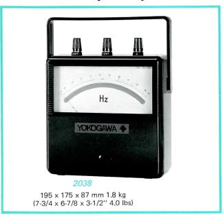
Model 2038 uses a frequency-to-DC current transducer which drives a high sensitivity moving coil type indicator. It features accurate frequency measurements without noticeable influence of line voltage fluctuation (50 to 300V) or waveform distortion.
