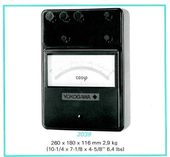
Model 2039 is used for measurement in single-phase and balanced three-phase circuits. From a phase discriminating circuit, the output of the built-in transducer produces a DC proportional to the phase between voltage and current to operate the DC indicator.
