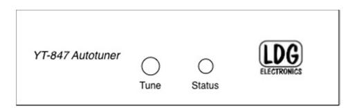
• **Tune Button:** Initiates either a memory tune or a full tune, and also toggles the tuner between "active" and "bypass" modes.
