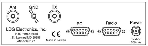
• **ANT connector:** Connect the 50-ohm coax antenna feedline to this standard SO-239 connector.
