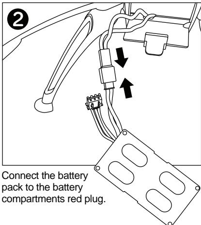
Connect the battery pack to the battery compartments red plug.
