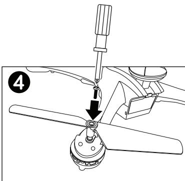
Replace the screw on the rotor. Repeat the process for any other damaged rotors.
