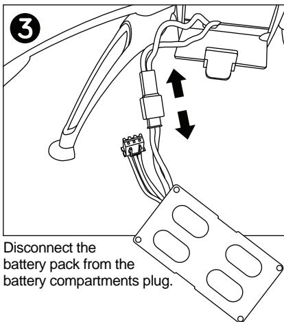
Disconnect the battery pack from the battery compartments plug.
