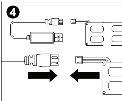
Connect the battery pack's white connector to the included USB charger then plug the USB to any powered USB port.
