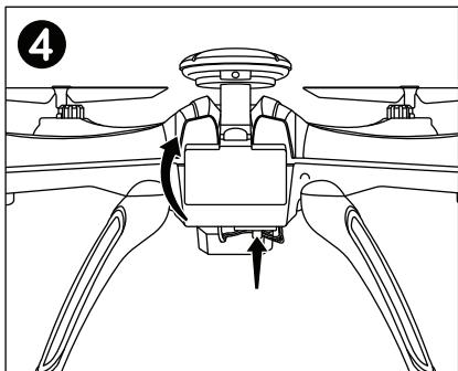
Close the battery compartment and switch on the drone power switch when ready to fly.
