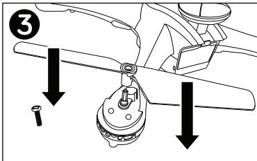
Place the correct A or B rotor on top of the peg.
