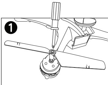
Use the included screwdriver to unscrew and remove the screw on the rotor.
