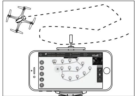
Only perform this action in an open area where there are no potential obstacles within a 25 foot radius. Start with simple routes and experiment to see what your drone can copy in the sky. Hard press any waypoint for over a second to edit the height. The drone will attempt to reach the specified height when at that waypoint. The default height for all waypoints is 98 feet. Press the "Up" icon to stop the flight and resume normal function.
