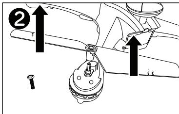
Remove the damaged rotor by lifting upward. Be sure not to misplace the screw.
