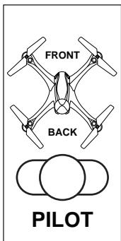
For Easy Mode to work properly you must launch the drone with the front of the drone facing away from the pilot as shown in the illustration to the left.
