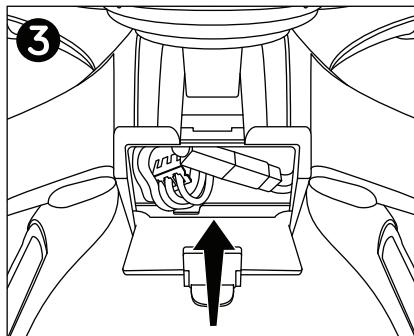
Put the battery pack into the battery compartment and arrange the connectors so everything fits inside.
