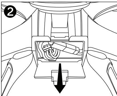
Gently pull the battery pack and connector cables out from the drone battery compartment.
