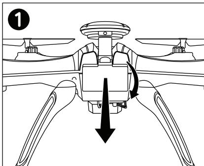
Make sure the drone power switch is in the OFF position. Pull the battery compartment door away from the drone and swing it open.
