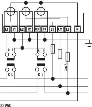
**(N) Neutral wire must be connected the meter**
