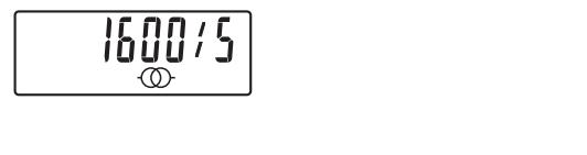
For the not MID certified meters to confirm the CT ratio you must reset the energy counters.
