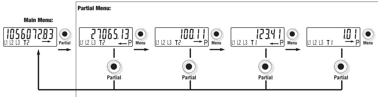
A pressure of 4 sec. of the "Menu key", in every page of the "Partial Counters" allows to enter in the zeroing menu of the "Partial Counters", and on the display appears "rESET".
