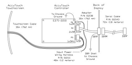
Figure 4.5 Touchscreen Cabling System for Internal Serial Controller
