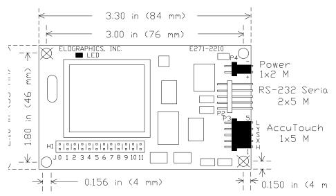
**Figure B.2** E271-2210 Serial Controller
