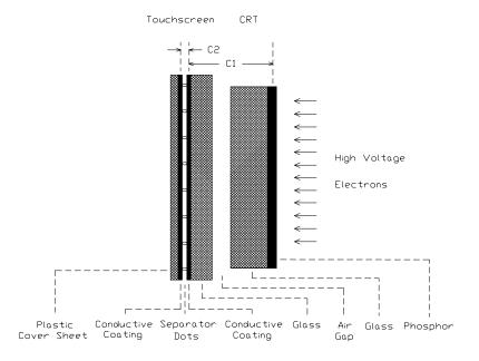
Figure 4.4 Side View of an AccuTouch Touchscreen Installation
