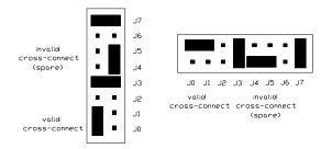
Figure B.1 SmartSet Controller Jumper Settings
