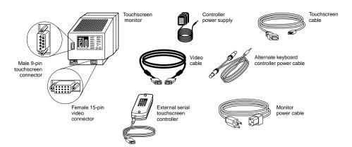
Figure 3.2 External Serial Controller Installation
