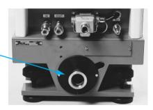
Disconnect the silencer from the pump exhaust connector by removing the clamping ring and the seal support ring. (Access via one of the side openings located at the bottom of the frame)
