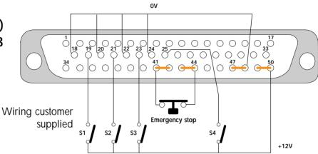
**NOTE**: The contact is considered to be closed if the DC voltage between 5 and 30 V is applied.
