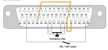
The remote control STOP button will stop the ADP, but it will restart as the push button is released.
