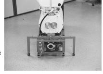
When pump is installed, the supports are stored, legs up, and fixed by means of two bolts. This kit is a part of modular pumps marked with a serial number upper than 973187. It can be fitted to retrofit on older pumps by ordering P/N 104527.
