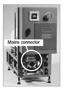
Mains connector is located on the electrical box lower face.
