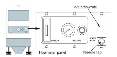
The water flow will be adjusted according to the processes with the needle tap (see section B120).
