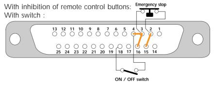
The remote control STOP button will stop the ADP, but it will restart as the push button is released.
