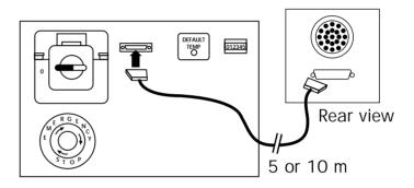
The remote monitoring unit is connected to the unit located on the frame via a 5 or 10 m cable, connected at the front. In this case, all controls are made from the remote unit. The frame-mounted unit only contains the main switch, the emergency stop and the monitoring system indicator lights.
