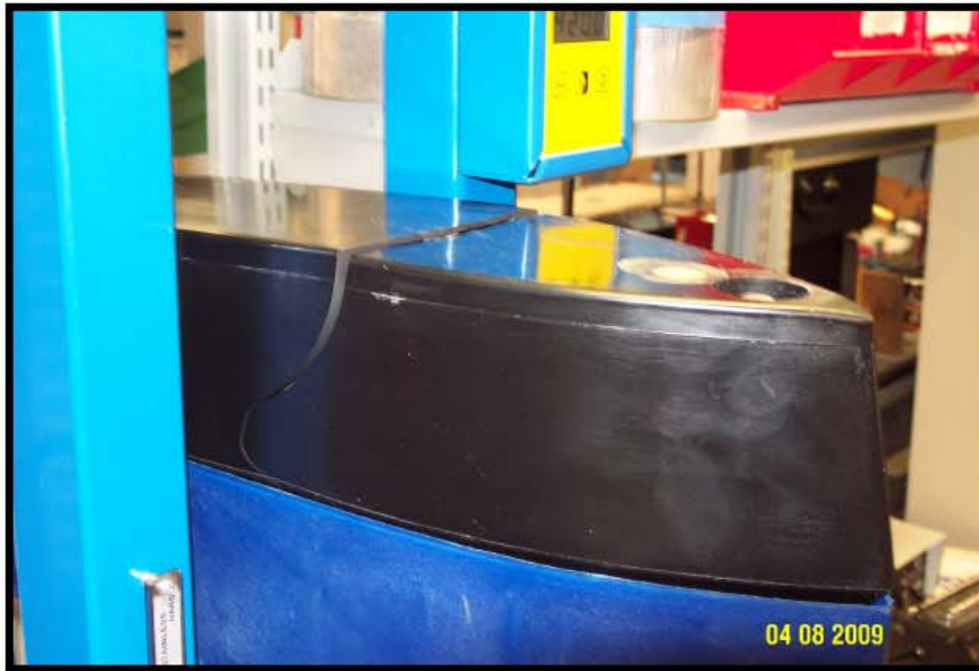
Figure 3: New R99 transducer failure at 4200 lbs (deflection 0.233") Failed with impact load from hammer
