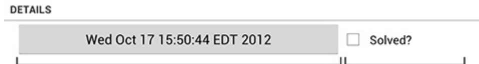
Figure 8.14 Extra space divided unevenly based on 2:1 layout_weight
