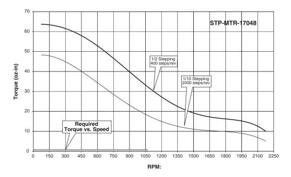
It looks like the STP-MTR-17048 stepping motor will work. However, we still need to check the load to motor inertia ratio:
