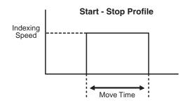
Equation ③:  $f_{SS}$  = indexing speed for start-stop profiles =  $P_{total} \div t_{total}$  $t_{total}$  = move time **Example 5:** What is the indexing speed to make a "start-stop" move with 10,000 pulses in 800 ms?
