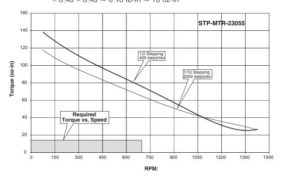
It looks like the STP-MTR-23055 stepping motor will work. However, we still need to check the load to motor inertia ratio:
