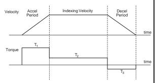
**Example 7:** What is the required torque to accelerate an inertia of 0.002 lb-in-sec<sup>2</sup> (motor inertia is 0.0004 lb-in-sec<sup>2</sup> and "reflected" load inertia is 0.0016 lb-in-sec<sup>2</sup>) from zero to 600 RPM in 50 ms?
