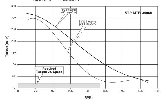
It looks like the STP-MTR-34066 stepping motor will work. However, we still need to check the load to motor inertia ratio:
