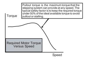
T<sub>run</sub> = constant motor torque requirement to run the mechanism due to friction, external load forces, etc.
