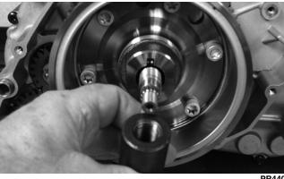
4. Install Magneto Rotor Remover Set and loosen the rotor/flywheel; then remove the crankshaft protector and rotor/flywheel from the crankshaft. Account for the flywheel key.
