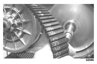
■NOTE: The arrows on the V-belt should point in direction of engine rotation (forward).
