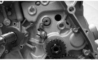
13. Remove the snap ring securing the output drive gear to the output shaft and remove the gear noting that the hub flange is directed toward the crankcase.
