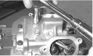
26. In a crisscross pattern starting from the center and working outward, tighten the cap screws (from step 25) to 8 ft-lb.
