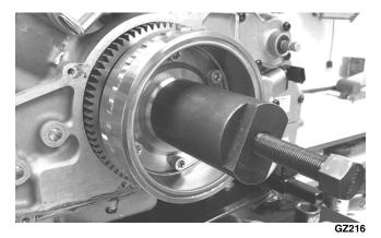
■NOTE: The puller has left-hand threads.
