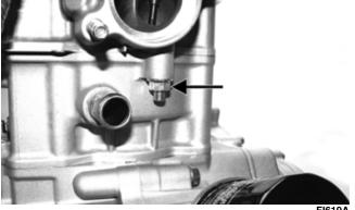
8. Remove the four cylinder head cap screws and washers. Note that the two cap screws on the right side of the cylinder head nearest the cam sprocket are longer than the two cap screws on the left (spark plug) side.
