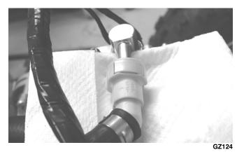
15. Install the air filter housing and secure to the throttle body with a hose clamp; then connect the IAT sensor connector.
