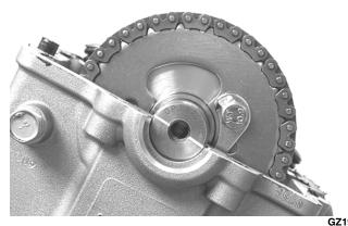
17. Keeping tension on the opposite cam chain, rotate the crankshaft until the second cap screw securing the sprocket to the camshaft can be installed; then install the cap screw (threads coated with red Loctite #271) and tighten to 10 ft-lb. Bend the tab to secure the cap screw.
