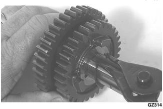
5. Install the reverse driven gear dog onto the countershaft and secure with a snap ring.
