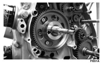
8. Install the rotor/flywheel and secure with the nut. Tighten to 107 ft-lb.
