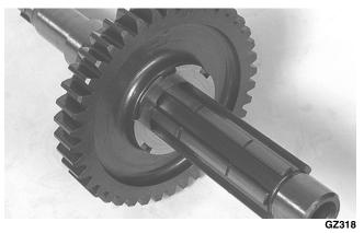
2. Install the low driven gear locking washer; then install the inner reverse driven gear washer.
