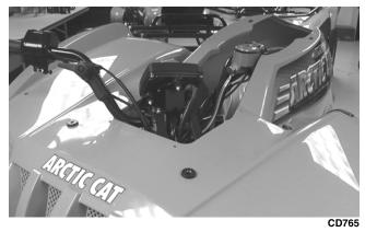
2. Connect the headlight connectors to the appropriate headlights and the front accessory plug wires to the accessory plug.
