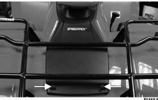
3. Remove four reinstallable rivets securing the steering post cover and remove the cover.
