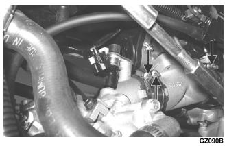
12. Connect the fuel injector, TPS connector (A), MAP sensor connector (B), and ISC valve connector (C).
