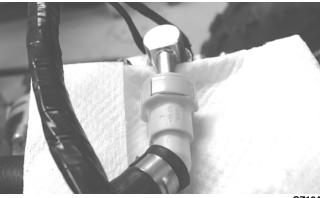
5. Disconnect the TPS connector (A), MAP sensor connector (B), and ISC valve connector (C) from the throttle body; then route the harness and connectors away from the engine.
