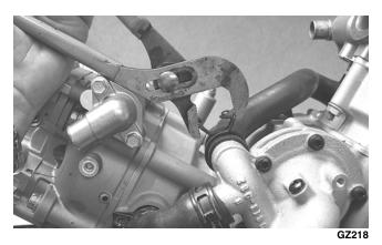
7. Remove the two cap screws securing the water pump to the crankcase; then remove the water pump. Account for an O-ring.
