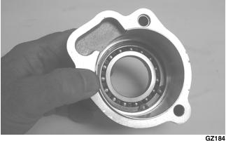
2. Using a suitable seal driver, install a new oil seal into the front of the input housing until the seal flush with the housing.
