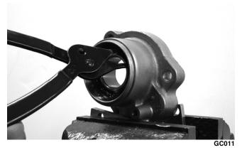
2. Install the input shaft seal making sure it is fully seated in the housing.
