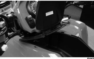
3. Remove the storage compartment box; then remove the seat.
