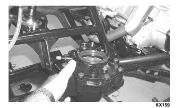
**Disassembling Input Shaft**
