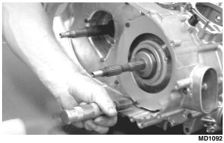
9. Remove the cap screws holding the clutch cover onto the right-side crankcase half. Note the positions of the different-lengthed cap screws for installing purposes.
