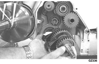
9. Engage the shift forks into the gear shift shaft and push the shift fork shaft into the crankcase.
