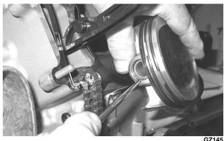
15. Using the Piston Pin Puller, remove the piston pin. Account for the opposite-side circlip. Remove the piston.
