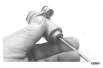
■NOTE: The adjuster shaft will be drawn into the tensioner as the adjuster screw is rotated clockwise. The adjuster shaft tension will be released in step 30.
