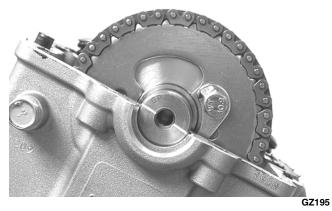
24. Rotate the crankshaft until the second cap screw securing the sprocket to the camshaft can be installed; then install the cap screw (threads coated with red Loctite #271) and tighten to 10 ft-lb. Bend the tab to secure the cap screw.
