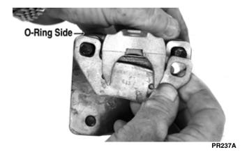
5. Remove the caliper holder from the caliper and discard the O-ring.
