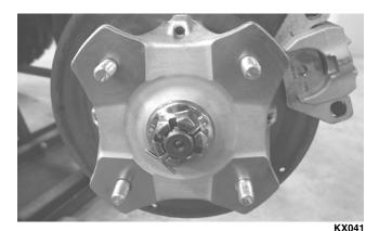
5. Remove the two brake calipers (right side only).
