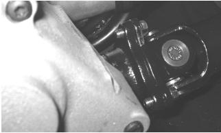
12. Remove the exhaust pipe springs at the muffler and remove the muffler. Account for the grafoil seal.
