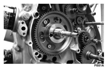
10. Remove starter idler gears and their respective shafts; then remove the starter motor. Account for an O-ring on the starter drive housing.
