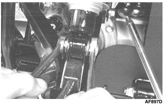
14. Remove the upper A-arm lock nuts and cap screws; then remove the A-arms.
