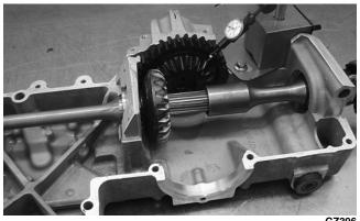
3. Firmly hold the bearings down and while rocking the drive bevel gear back and forth, note the maximum backlash reading on the gauge.
