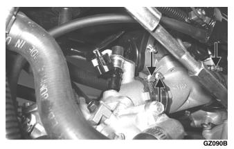
Disconnect the fuel injector wiring connectors; then remove the intake manifolds leaving the injectors installed.
