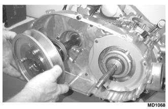
8. Using an impact screwdriver, remove the three Phillips-head cap screws holding the air intake plate. Remove the air intake plate.
