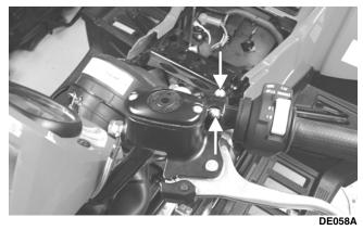
2. Using two new crush washers, connect the banjo-fitting to the master cylinder; then secure with the banjo-fitting bolt. Tighten to 20 ft-lb.
