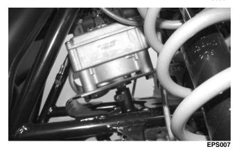
3. Install the tie rods and secure with the slotted nuts. Tighten to 30 ft-lb; then install new cotter pins.
