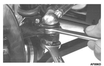
10. Remove the upper ball joint cap screws taking care not to strip the threads on the ball joint shaft; then using a rubber mallet, tap the end of the axle and free it from the knuckle assembly.
