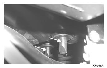
2. Replace any drain that is cracked or shows any signs of hardening or deterioration.
