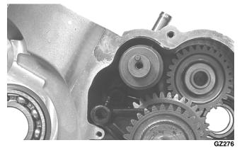
6. Remove two cap screws securing the oil pump in the crankcase and remove the oil pump.
