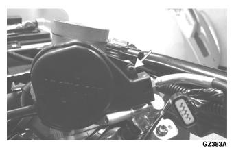
6. Use tape to cover and seal the intake opening.
