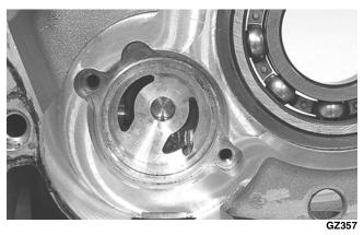
3. Inspect the gerotor set for scoring, discoloration, or cracks; then using a feeler gauge, check the inner to outer rotor clearance. If measurements exceed specifications, the gerotor set must be replaced.
