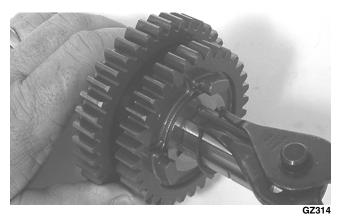
5. Remove the reverse driven washer; then remove the low driven gear locking washer.
