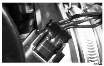
2. Remove the screw securing the TPS to the throttle body and remove the TPS.
