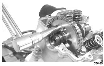
25. Rotate the crankshaft until the first cap screw (from step 23) can be addressed; then tighten to 10 ft-lb. Bend the tab to secure the cap screw.
