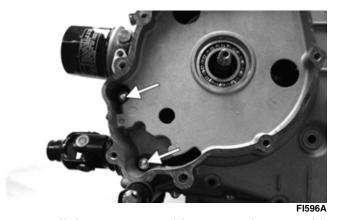
10. Install the water pump drive gear and secure with the nut. Tighten to 28 ft-lb.
