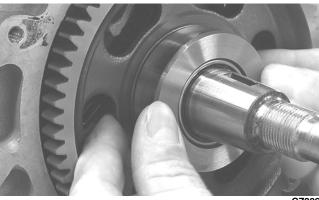
11. Place the key into the keyway in the crankshaft; then wipe all oil from the crankshaft surface and rotor/flywheel bore and install the rotor/flywheel onto the crankshaft aligning the keyway with the key. Secure with the nut and tighten to 107 ft-lb.
