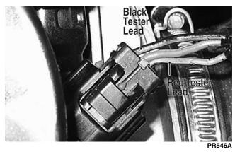
8. Select the DC Voltage position on the meter and turn the ignition switch to the ON position. The meter should read approximately 0.6 DC volt with the throttle closed and approximately 4.0 DC volts with the throttle in the full-open position.
