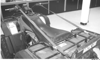
6. Measure the distance from the inside of each front rim to the lower frame tube.
