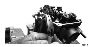
■NOTE: At this point, oil the camshaft bearings, cam lobes, and the three seating journals on the cylinder head.
