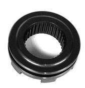
4. Remove the snap ring securing the reverse driven gear and washer; then remove the washer and gear.
