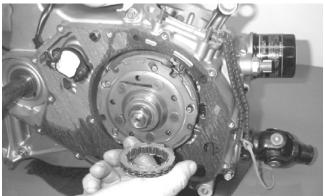
12. Remove the left-hand threaded nut holding the centrifugal clutch assembly.
