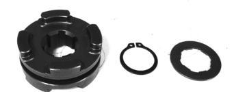
5. Remove the circlip securing the high driven gear; then remove a washer, the high driven gear along with the bearing and bushing, and remove the high driven washer.
