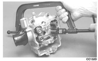
2. Remove the valve seal and the lower remaining spring seat. Discard the valve seal.
