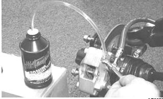
2. Place an absorbent towel around the connection to absorb brake fluid. Remove the banjo-fitting from the master cylinder. Account for two crush washers and a banjo-fitting bolt.
