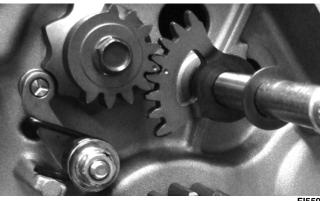
12. Remove the shift detent cam arm and spring.
