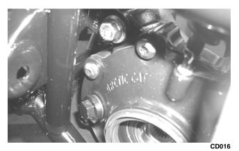
20. Free the differential assembly from the frame mountings; then shift the differential assembly forward enough to disengage the front driveshaft from the output yoke.
