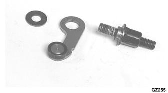
6. Install the shift cam stopper spring onto the shift cam stopper and secure with a flat washer and flange nut. Tighten to 8 ft-lb.
