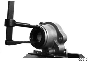
6. Remove the snap ring securing the input shaft bearing; then place the pinion housing in a press and remove the bearing.
