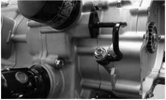
4. Remove the water pump drive gear; then remove the speed sensor housing assembly. Account for two alignment pins, a gasket, and two seal wash-
