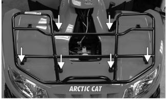
6. Remove the side panels by pulling on them to release the tabs from the body; then remove the screws securing the rear of the front panel to the frame.
