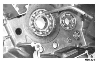
■NOTE: If heating the bearing is not possible, the crankshaft can be installed using a crankshaft installer.
