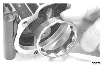
2. Using the Pinion Gear/Shaft Removal Tool and a hammer, remove the pinion gear from the gear case housing.
