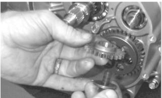
16. Remove the snap ring holding the oil pump driven gear.
