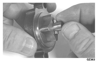
3. With the outer rotor reference dot directed toward the oil pump cover, install the rotor onto the inner rotor.
