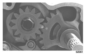
9. Apply grease to the lips of the shift shaft seal in the shifter housing; then using a new gasket, install the shifter housing and secure with the cap screws.
