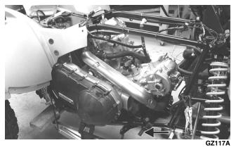
22. Fold the front drive line up and secure against the front of the engine; then lift the engine clear of the mountings and remove from the right side of the frame.
