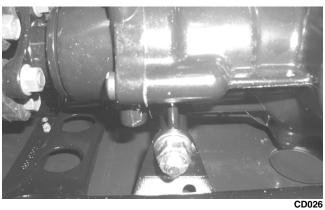
19. Remove the upper differential mounting cap screws.
