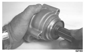
2. Remove the clutch pack from the clutch basket; then remove the snap ring securing the clutch basket (A) to the input shaft (B) and remove the clutch basket.
