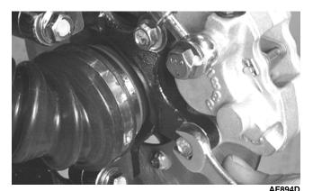
8. Remove the tie rod cotter pins and discard the pins.
