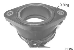
11. Use tape to cover and seal the intake opening.
