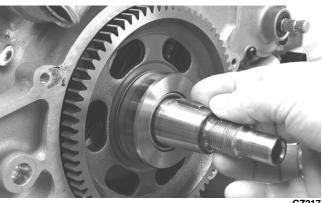
5. With the flywheel key removed, remove the starter ring-gear and spacer washer.
