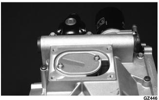
2. Remove the cap screws securing the lower crankcase to the upper crankcase halves; then using a rubber hammer, free the lower crankcase and remove. Account for two alignment pins.
