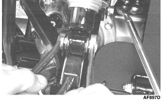
8. Secure the tie rods with the lock nuts. Tighten to 30 ft-lb; then install and spread the cotter pins.
