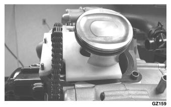
3. Lubricate the inside wall of the cylinder; then using a ring compressor, compress the rings and slide the cylinder over the piston. Route the cam chain up through the cylinder cam chain housing; then remove the piston holder and seat the cylinder firmly on the crankcase.
