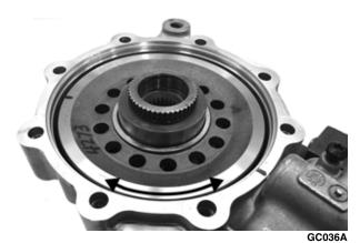
3. Install the bearing flange onto the gear case cover making sure the alignment/locating pin engages the locating hole in the cover; then make sure the bearing flange is completely seated in the cover.
