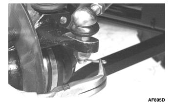
9. Remove the tie rod lock nuts.
