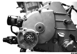
12. Install the water pump cover with a new O-ring and secure with the four cap screws. Tighten to 8 ft-lb.
