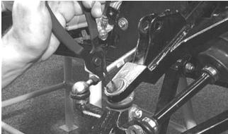
2. Install the A-arm assemblies into the frame mounts and secure with the cap screws. Only finger-tighten at this time.
