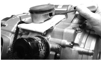
14. Using Piston Pin Puller, remove the piston pin. Account for the opposite-side circlip. Remove the piston.
