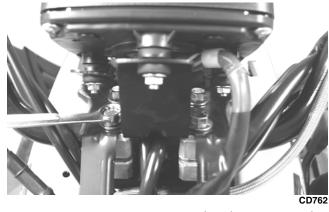
7. Remove two cap screws securing the upper steering post bearing to the frame. Account for two housings.
