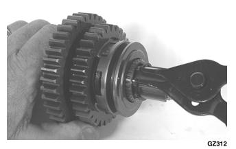
3. Remove the reverse driven gear dog.
