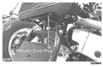
18. Remove the bleed screw from the water pump; then after coolant has drained, apply compressed air to the bleed opening to purge the remaining coolant from the system. Install the bleed screw and radiator drain plug and tighten securely.
