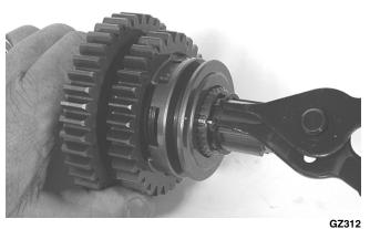
6. From the opposite end of the countershaft, install the high/low driven gear dog (A), thrust washer (B), bushing (C), bearing (D), high/low driven gear (E), and spacer washer (F).
