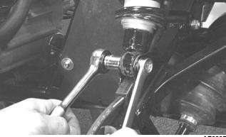
4. Compress the shock absorber spring, remove the retainer, and remove the spring.
