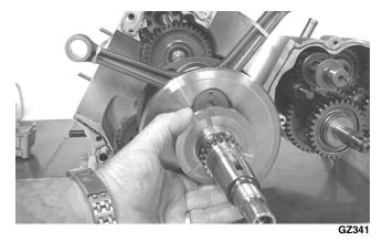
3. Install the two alignment pins; then apply a thin bead of silicone sealant to the crankcase mating surface.
