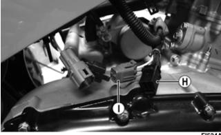
8. Connect the engine ground cable to the starter mounting flange and secure with a cap screw tightened to 8 ft-lb.
