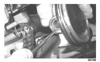
Place the two alignment pins into position. Place the cylinder gasket into position; then place a piston holder (or suitable substitute) beneath the piston skirt and square the piston in respect to the crankcase.
