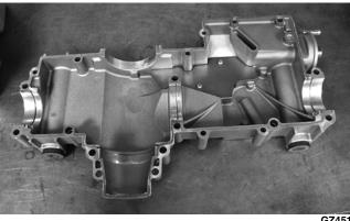
9. Carefully place the lower crankcase cover onto the joined crankcase halves; then secure with the cap screws. Tighten the 6 mm cap screws to 8 ft-lb and the 8 mm cap screws to 20 ft-lb.
