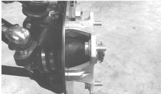
14. Remove two cap screws securing the lower steering post bearing flange to the frame; then remove the steering post.
