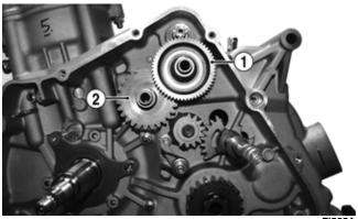
7. Install the starter clutch gear onto the crankshaft; then install the rotor/flywheel key in the crankshaft.
