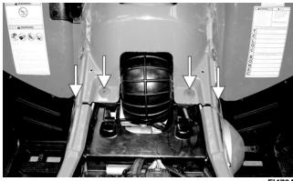
7. Remove the left and right footwells; then remove the shift knob. Remove the shift lever pivot axle nut and remove the axle and shift lever. Account for a spring and two O-rings.
