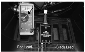
4. Adjust the TPS until a reading of 0.68 DC volt is obtained; then tighten the screw securely. Open and close the throttle and determine the reading returns to 0.68 DC volt. Readjust as necessary.
