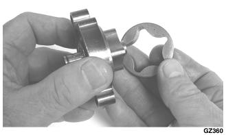
4. Place a new O-ring seal on the outside of the oil pump cover. The oil pump assembly is now ready for assembly into the crankcase.
