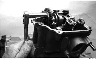
18. Rotate the crankshaft until the second cap screw securing the sprocket to the camshaft can be installed; then install the cap screw (threads coated with red Loctite #271). Tighten to 11 ft-lb; then bend the tab to secure the cap screw.
