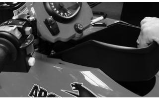
4. Remove the ignition switch retaining ring and two reinstallable rivets securing the instrument pod; then remove the instrument pod.
