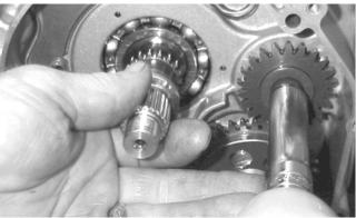
7. Install the clutch shoe assembly on the crankshaft; then install the flange nut (left-hand thread) (coated with red Loctite #271). Tighten to 147
