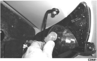
9. Rotate the handlebar to the full-left position; then lift and slide the panel to the rear and lift the rear up to clear the handlebar.
