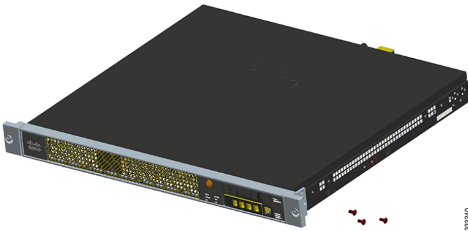
Figure 6 Install Die-Cast Brackets with Three Screws
