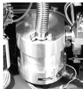
LDS valve (connected to the TMP rear)
