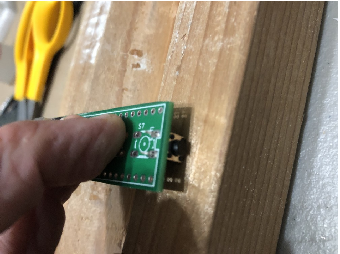
A good way to align before soldering
