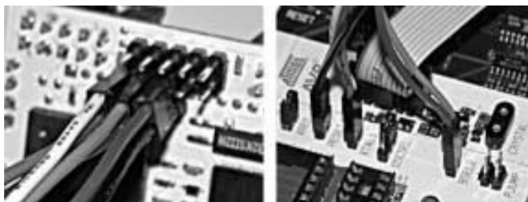
Figure 3-5. Reset, BSEL2 and XTAL1 cables
