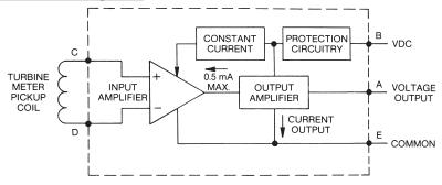
The turbine meter pickup coil is connected to screw terminals C and D, which are connected to the primary of the input transformer. The transformer secondary drives the operational amplifier in a differential mode, with a small amount of hysteresis provided by resistors R5 and R6.
