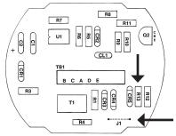
In addition, a non-linear resistor CL1 absorbs transient energy spikes greater than 39 volts and CR2 protects the circuitry against inadvertent reversal of the power input polarity.
