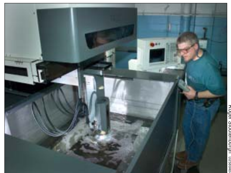
Tool and Instrument Maker Chris Manning tests out the new Mitsubishi FA-30 traveling wire electrical-discharge machine, the largest of its type on the U.S. east coast.
