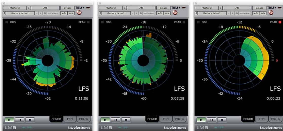
Fig 3, Loudness meter adhering to ITU-R BS.1770. Left: Feature film (Pirates of the Caribbean): Low Loudness Consistency typical of film. Center: Broadcast (German national broadcaster): Consistency suitable for broadcast. Right: Pop music (Madonna): Overly high Consistency typical of pop. Generates listener fatigue.
