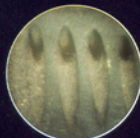
Coolant holes on turbine blade as seen through Lenox flexible borescope.
