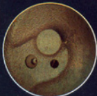
Diesel injector nozzle as seen through Lenox flexible borescope.
