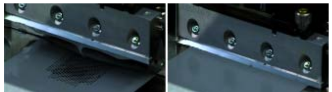
Figure 4: Flooding the stencil and removing the excess material afterwards to achieve the best possible printing results
