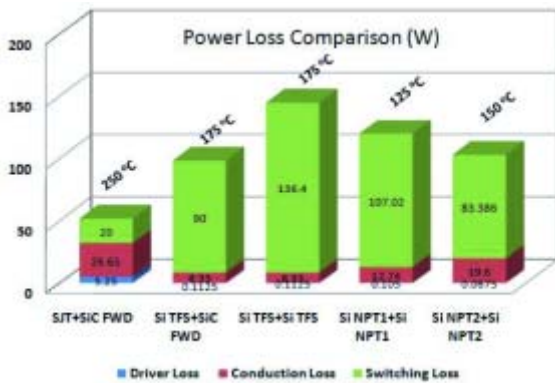
Figure 6 : Power loss comparison of SiC SJT and Si IGBT co-packs at their maximum operating temperature
