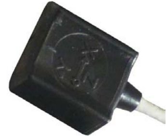
Tri-axial accelerometer uses 3 channel inputs
