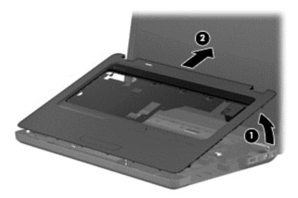
NOTE: The TouchPad is glued to the top cover and is included with the top cover spare part.
