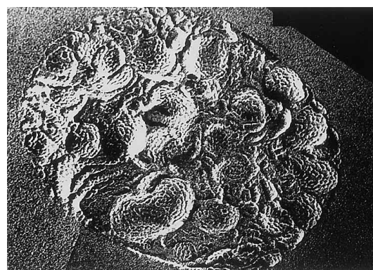
Fig. 3. Freeze-Fracture Electron Micrograph of EggPC/30 mol% DSPE-PEG2000 LUV
