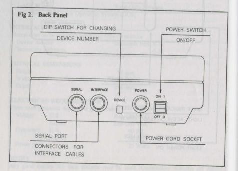
After plugging the power supply into the disk drive and a suitable outlet, find the black cable that goes from the disk drive to the computer. It is called a serial bus cable to describe the way the computer, and other accessories communicate with each other through its wires. It has an identical 6-pin DIN connector at each end, which like the power connector can only go in one way—with the dimple in the side of the plug facing up.
