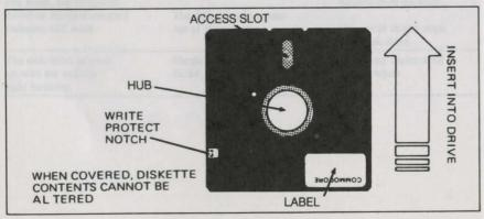
Fig.4. Position for Diskette Insertion
