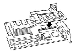
2. Press the EpsonScript board in firmly until it stops secure the EpsonScript board with the screws that come with it.
