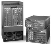
scalable system in the industry, each router offers the ability to bring DS0 to OC-48 WAN connectivity, and 10-Mbps Ethernet to 10-Gigabit Ethernet LAN connectivity to the Internet data center, metropolitan aggregation, WAN edge aggregation, and enterprise networking applications. The Cisco 7600 Internet Router is an important component of Cisco's end-to-end IP+Optical offerings, helping service providers break through service and bandwidth barriers to increase new revenues and profits.
