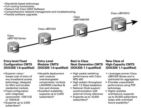
\* Typical deployment scenario for data; actual numbers vary depending on network/service loading, etc.
