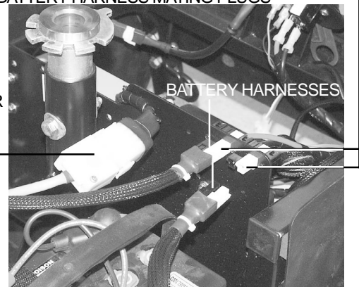
Figure 12A. Disconnect Battery Harnesses
