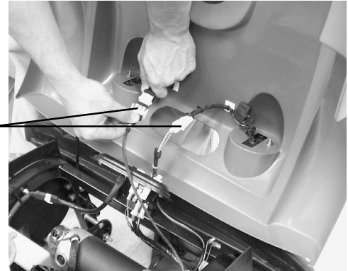
Figure 12. Disconnect Lighting Harnesses
