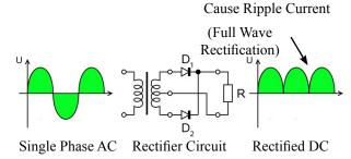
Form factor is the ratio of  $I_{rms}$  to  $I_{dc}$  and indicates how close the driving voltage is to pure DC. The form factor for a DC battery is 1.0. The higher the form factor is above 1.0, the more it deviates from pure DC. The Form Factor Table shows examples of commonly used voltages.
