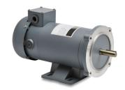
IronHorse 56C frame PMDC motors are available from 1/3 hp to 2hp. All models have a TEFC or TENV rolled steel frame, cast aluminum end bell and removable mounting bases. Motors have easy-access brushes.
