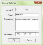
Press the OK button to write the new configuration to the GS-EDRV.
