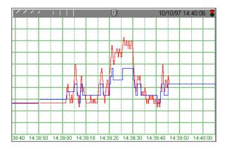
The Citadel database also uses **Deviation** as the criteria which triggers logging of new historical data to disk. See Chapter 7, *Logging Data and Events*, in the *LookoutDirect Developer's Manual* for more information on logging data.
