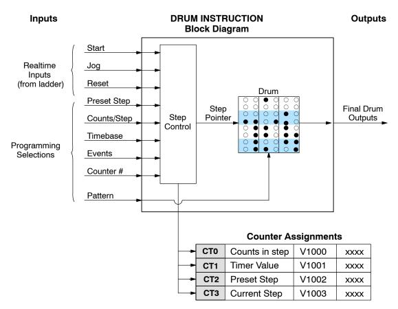
The drum instruction accepts several inputs for step control, the main control of the drum. The inputs and their functions are:
