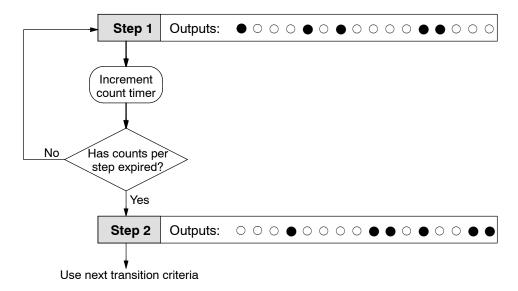
The drum stays in Step 1 for a specific duration (user-programmable). The timebase of the timer is programmable, from 0.01 seconds to 99.99 seconds. This establishes the resolution, or the duration of each "tick of the clock". Each step uses the same timebase, but has its own unique counts per step, which you program. When the counts for Step 1 have expired, then the drum moves to Step 2. The outputs change immediately to match the new pattern for Step 2.
