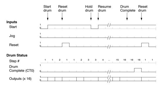
When the drum completes the last step (Step 16 in this example), the Drum Complete bit (CT0) turns on, and the step number remains at 16. When the Reset input turns on, it turns off the Drum Complete bit (CT0), and forces the drum to enter the preset step.
