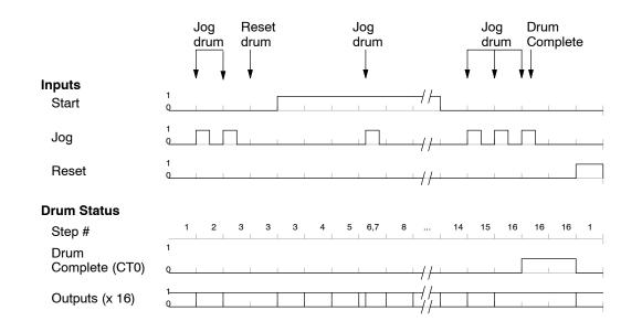
Self-Resetting Applications often require drums that Drum automatically start over thev once complete a cycle. This is easilv accomplished, using the drum complete bit. In the figure to the right, the drum instruction setup is for CT0, so we logically OR the drum complete bit (CT0) with the Reset input. When the last step is done. the drum turns on CT0 which resets itself to the preset step, also resetting CT0. Contact X2 still works as a manual reset.
