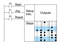
The timing diagram below shows an arbitrary timer drum input sequence and how the drum responds. As the CPU enters Run mode it initializes the step number to the preset step number (typically it is Step 1). When the Start input turns on the drum begins running, waiting for an event and/or running the timer (depends on the setup).
