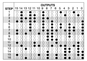
**Output Sequences** The mechanical drum sequencer derives its name from sequences of control changes on its electrical outputs. The following figure shows the sequence of On/Off controls generated by the drum pattern above. Compare the two, and you will find that they are equivalent! If you can see their equivalence, you are well on your way to understanding drum instruction operation.
