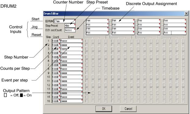
The Event Drum features 16 steps and 16 discrete outputs. Step transitions occur on timed and/or event basis. The jog input also advances the step on each off-to-on transition. Time is specified in counts per step, and events are specified as discrete contacts. Unused steps must be programmed with "counts per step" = 0, and event = "K0000". The discrete output points may be individually assigned.
