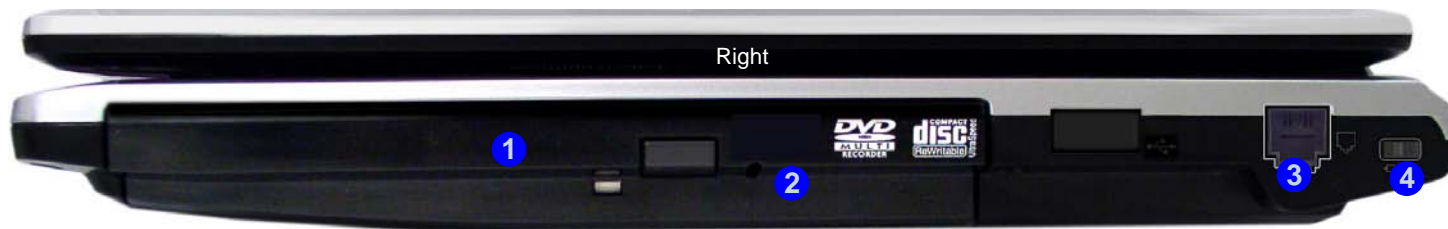
Figure 5 Right Side View 1. Optical Device Drive Bay 2. Emergency Eject Hole 3. RJ-11 Phone Jack 4. Security Lock Slot
