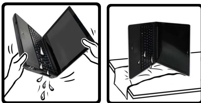
Figure 2 - Drain any Liquid to the Right Side and Rest the Computer on the Right Side to Dry
