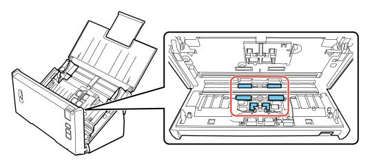
5. Wipe off any dust or dirt on the pickup rollers.
