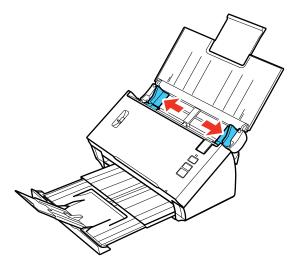
4. Load one plastic card horizontally in the input tray as shown, sliding it in until it meets resistance. Make sure the printed side is facedown and top edge first.
