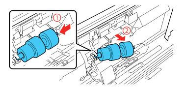
12. Pull the release tab on the separation roller and remove it from the spindle.
