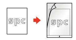
• If the original is larger than the carrier sheet, fold it in half with the sides to be scanned facing out. Position the right side of the original faceup with the top facing the arrow on the sheet.
