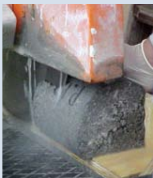
Preparing (top) and placing (bottom) RCC prisms for freeze-thaw testing
