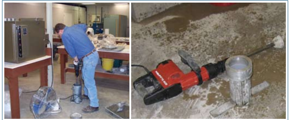
Figure 4-5. Molding RCC cylinder with vibrating hammer
