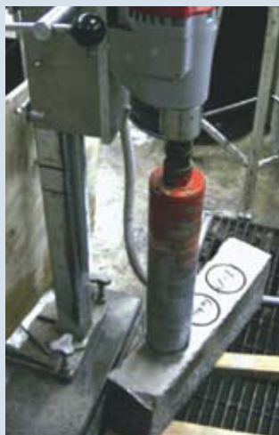
Bond strength test core
