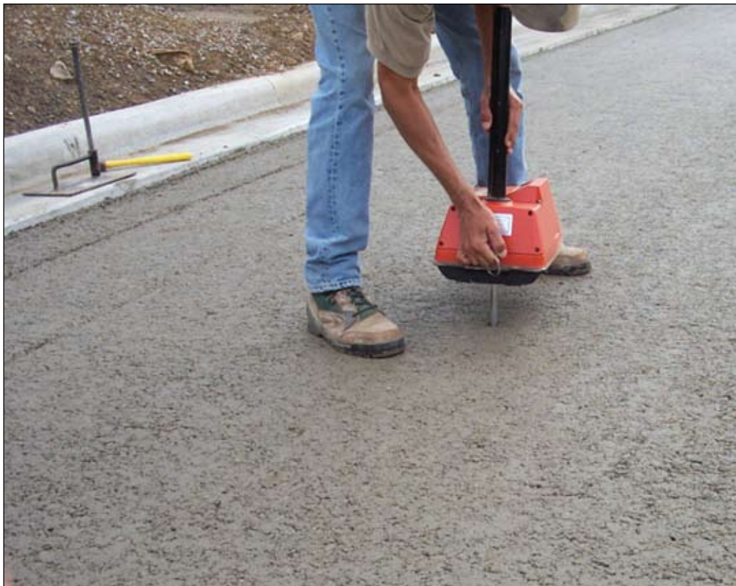
Figure 7-3. Checking density using a single-probe nuclear gauge
