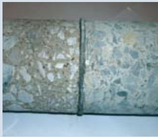
Pavement core showing multi-layer system with geotextile fabric layer
