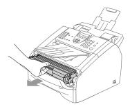
3 Hold down the lock lever on the left and pull the toner cartridge out of the drum unit. Take out the jammed paper if there is any inside the drum unit.
