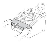
Pull out the drum unit and toner cartridge assembly.
