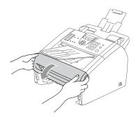
4 Pull out the drum unit and toner cartridge assembly. The jammed paper may be pulled out with the toner cartridge and drum unit assembly, or this may release the paper so you can pull it out of drum unit or the paper tray opening.
