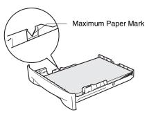
5 Put the paper tray firmly back in the machine. Lift the ADF document output support and unfold the output paper tray support flap before you use the machine.
