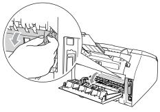
Drull the jammed paper out of the fuser unit. If the jammed paper cannot be pulled out easily, push down the blue tab with one hand as you gently pull out the paper with the other hand.
