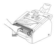
Clean the primary corona wire inside the drum unit by gently sliding the blue tab from right to left several times.
