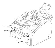
Using both hands put one sheet of paper in the manual feed slot until you feel the front edge of the paper touch the paper feed roller. Let go of the paper when you feel the machine feed the paper in a short distance.
