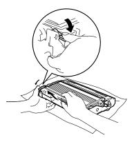
4 Put the toner cartridge back into the drum unit until you hear it lock into place. If you put it in properly, the lock lever will lift automatically.
