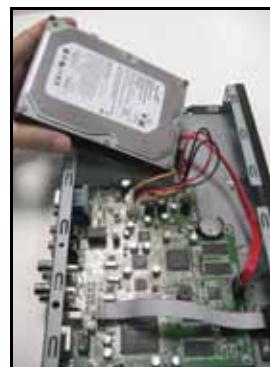
Figure 27.3 Carefully remove the HDD from housing.
