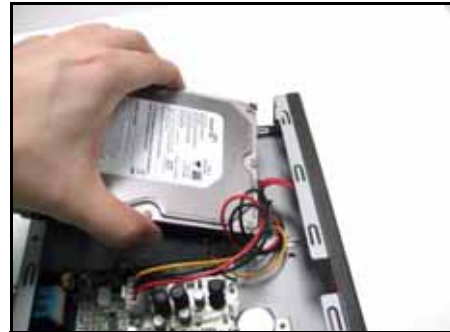
Figure 27.5 Insert the drive carefully
