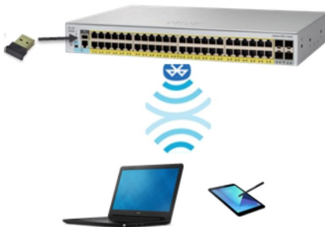
Figure 4. Over-the-air switch access using Bluetooth
