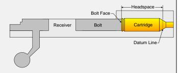
Note that excessive headspace, which is excessive linear endplay of a cartridge in the chamber with the bolt closed, allows movement of the case during firing, which can cause dangerous case stretching, case separation and gas leakage.
