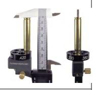
**Step 7:** Measure the other four cases, record the measurements and calculate the average. <u>Remember:</u> repeatability is important when taking measurements.
