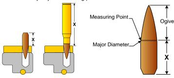
This measurement then allows you to adjust your seating die to achieve the optimum distance from the bullet ogive to the lands of the rifle. Obtaining the best bullet seating depth for a specific bullet to be used in a specific firearm significantly improves the accuracy of your loaded rounds.
